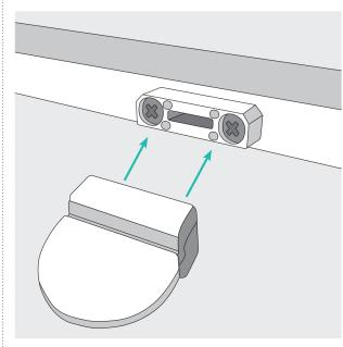
Secure handle to blind by pushing onto the mounting block already screwed to the operating rail.
