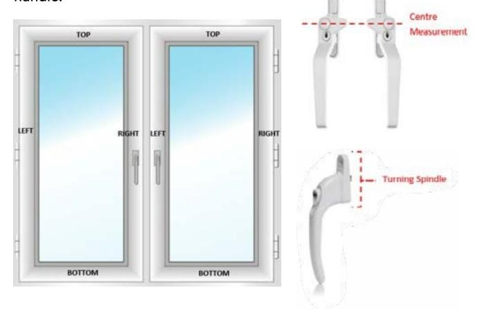
If the handle is located on the right or the left side of your window, you will need to measure from the beading at the top of the window to the centre of your handles turning spindle.
