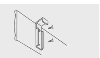
Hook valance clip with valance attached onto the top of the headrail.
